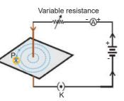
The magnetic field strength decreases with increase of distance from the current carrying conductor.
